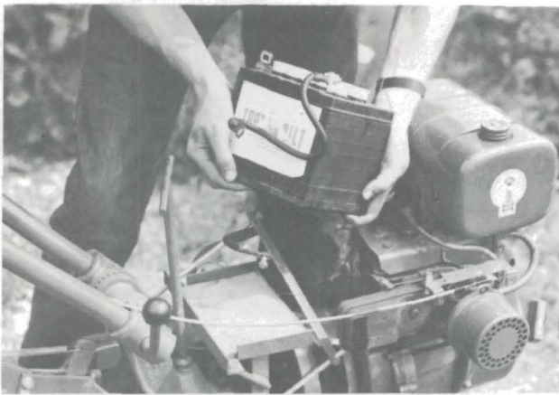
Photo 5: Be sure the battery on electric starting units is charged and in good condition (a weak battery may freeze during cold weather). Disconnect battery and store in a cool, dry place. Temperatures best for storage range from 10° to 45°F., as long as the battery retains its charge. A weak battery can freeze and rupture.
