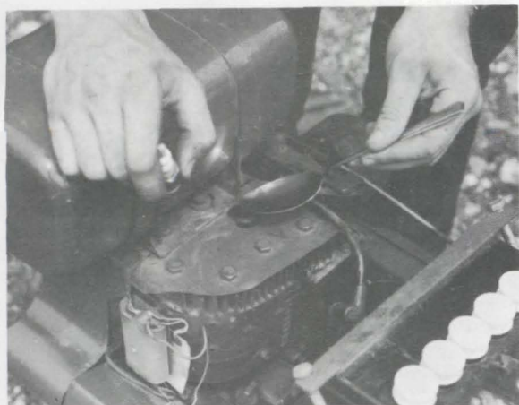
Photo 3: Remove spark plug, then pour a tablespoon of clean engine oil into spark plug hole. Pull the recoil starter. Clean and replace the spark plug, but don't connect the spark wire until springtime. Now distribute the oil by slowly pulling the starter until you feel compression.
