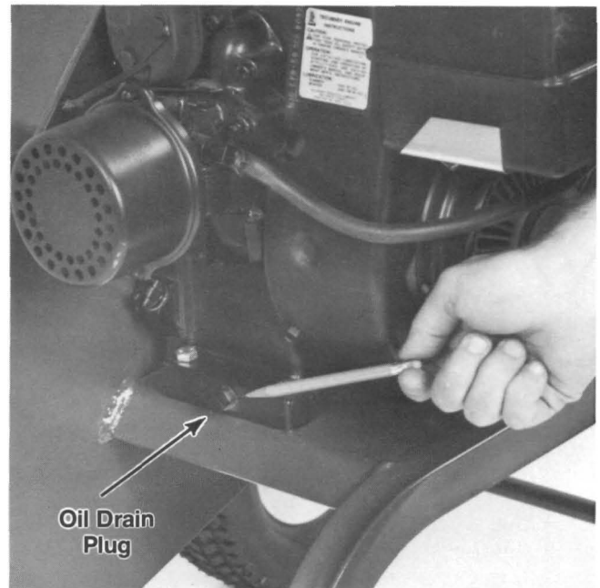
(Photo 5-2) Left-side oil drain plug on Tecumseh engine.
