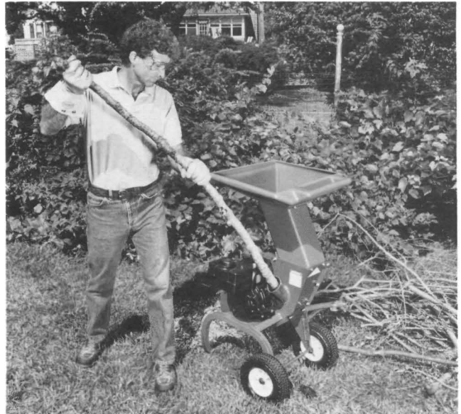
(Photo 4-2) Feed material into chipper at proper angle, and rotate branches. Do not overload the chipper.
