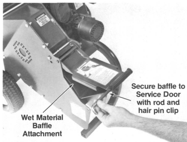
(Photo 3-8) Attach other end of Baffle Attachment to the Service Door using a rod and hair pin clip. Close the Service Door and secure it with a rod and hair pin clip.
