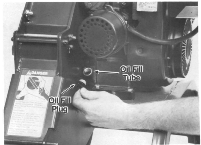
(Photo 2-3) Turn Oil Fill Plug counterclockwise to remove it from the Oil Fill Tube. If tight, use a screwdriver blade as a lever between the two posts.
