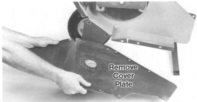
(Photo 5-10) Remove 12 bolts securing cover plate to the main housing. Take cover plate off.
