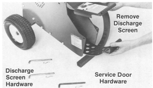
(Photo 5-8) Remove the Discharge Screen. First, pull out the two hair pin clips and slide out the two rods securing the discharge screen. While holding up the service door slide the screen out and put it aside with its hardware. Note how the screen ends are different — during reassembly, the end that's bent back the most goes in first.
