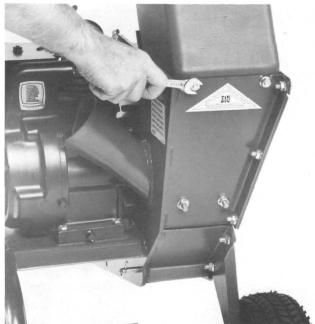
(Photo 2-2) Double-check hardware tightness all around the equipment — especially the shredder hopper.
