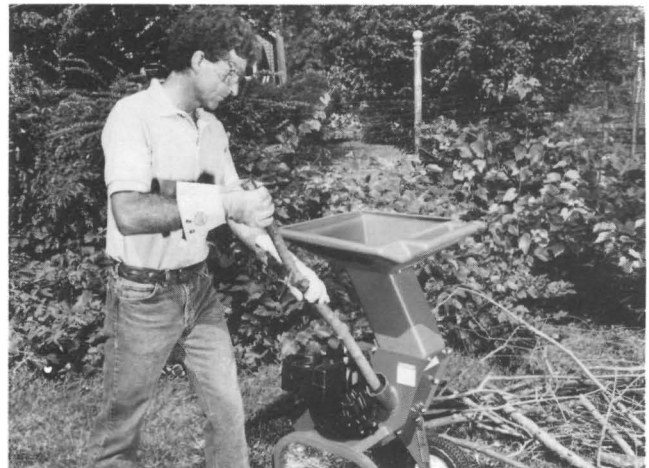
(Photo 4-3) Hold branches firmly; feed in smoothly.
