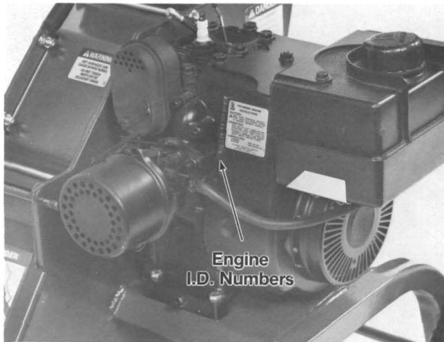
(Photo 5-1) Location of Tecumseh engine I.D. numbers.
