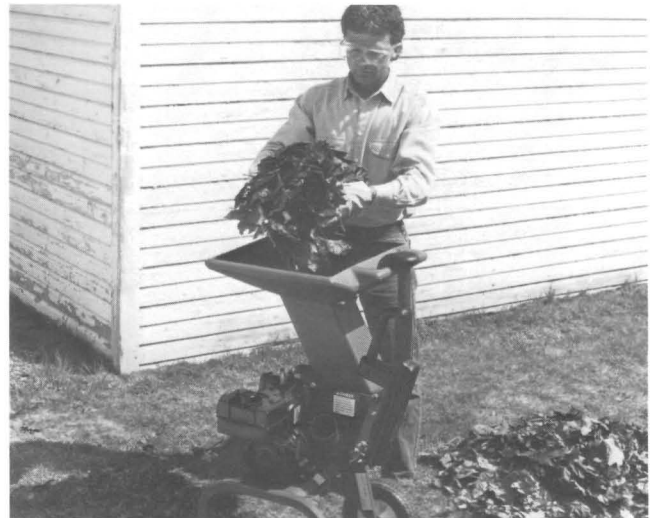
(Photo 4-6) Feed materials in steadily and slowly, but don't overload the shredder. Your Leaf Tamper can hang conveniently on the shredder handle, ready for use.
