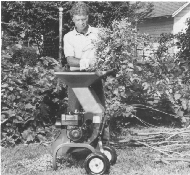
(Photo 4-5) When using the Shredder, stand 1-to-2 feet away from the top-loading hopper and release materials into it.
