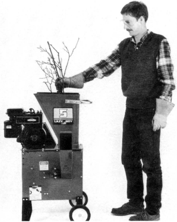
PHOTO 4-3: Feeding material into the Shredder Hopper. Stand a foot or two away from the hopper opening and keep your arms and hands parallel to, and several inches above the top edge of the hopper.
