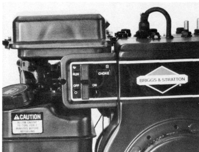
PHOTO 3-6: OFF/ON lever and Choke Control lever.
