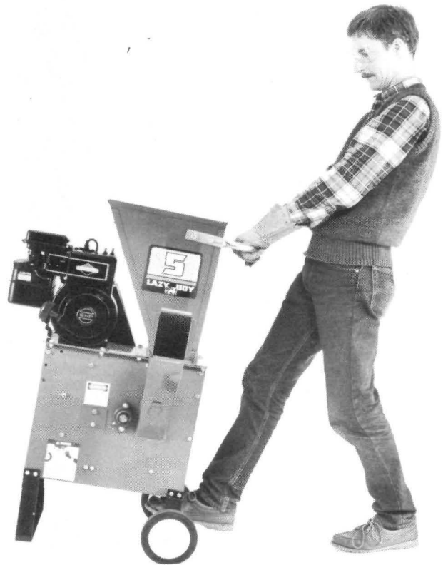
PHOTO 4-1: Moving the chipper/shredder. Never move the machine while the engine is running.
