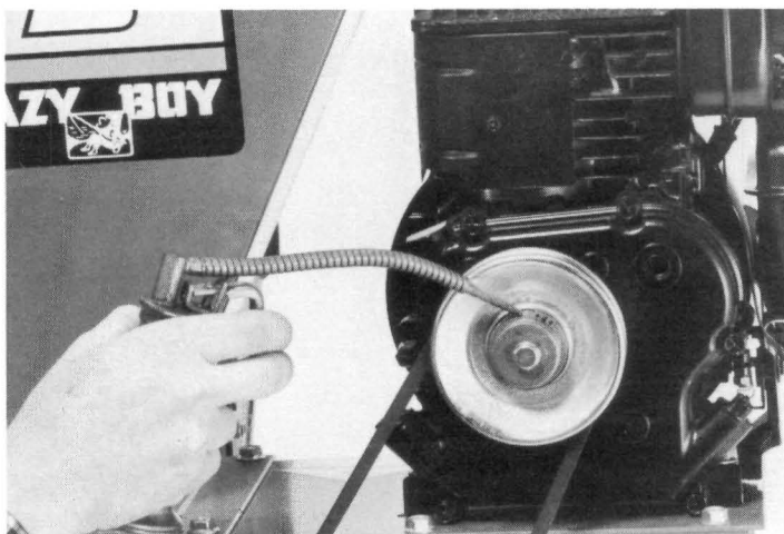
PHOTO 5-4: Apply oil to rotating ring on centrifugal clutch. Be sure to reinstall the belt guard before operating the unit.
