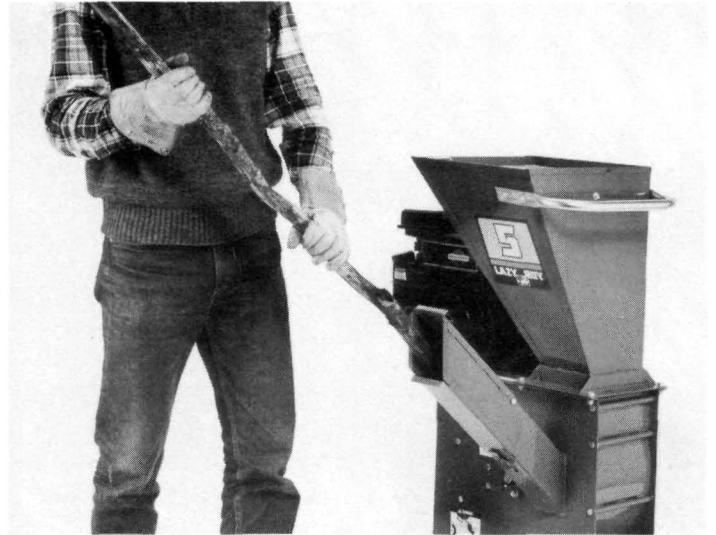
PHOTO 4-2: Feeding a branch into the chipper chute. Keep arms perpendicular (at 90°) to the branch.
