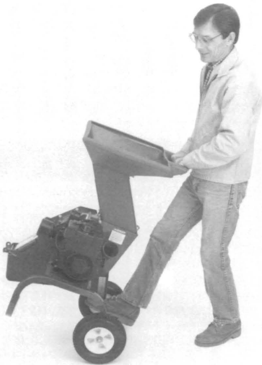
(Photo 4-1) To move your Chipper/Shredder, plant one foot on the axle, tilt equipment back with both hands until "balance point" is reached, then push or pull your equipment to a work area. Engine must be OFF.
