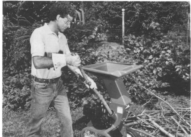
(Photo 4-3) Hold branches firmly; feed in smoothly.
