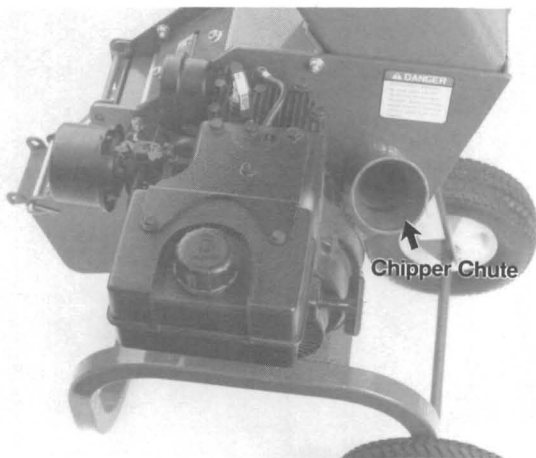
(Photo 3-3) The Chipper Chute is for processing larger, heavier branches (½”-to-2” in diameter).
