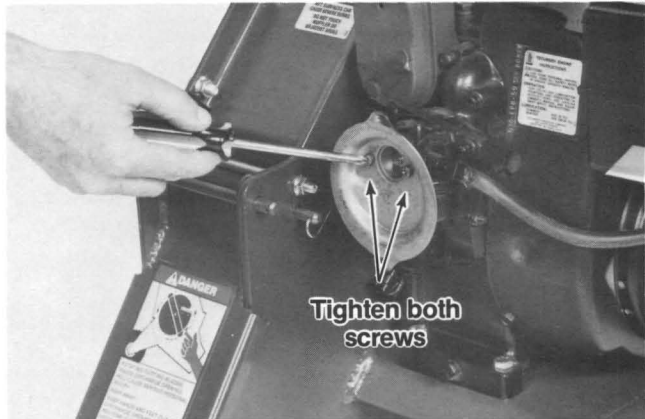
(Photo 5-4) Tecumseh air cleaner back mounting plate. Check to see both screws are secure.
