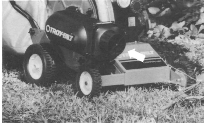
Photo 4-16: Vacuum Inlet Cap.
