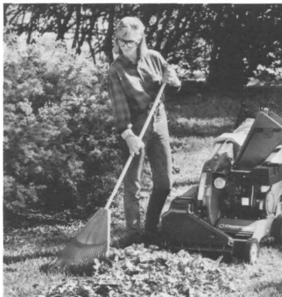
Photo 3-4: Rake material directly into Rake-In Tray.
