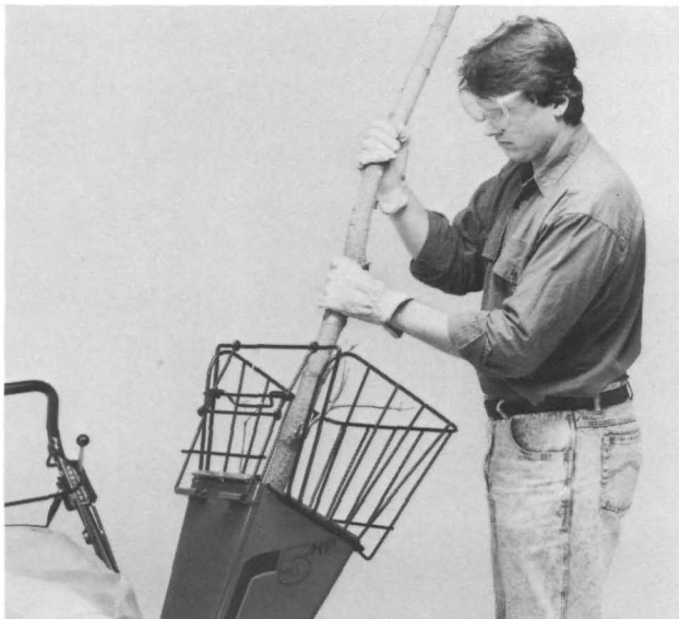
Photo 4-14: When feeding branches into the chipper chute, keep your arms perpendicular (at 90° angle) to the branch.
