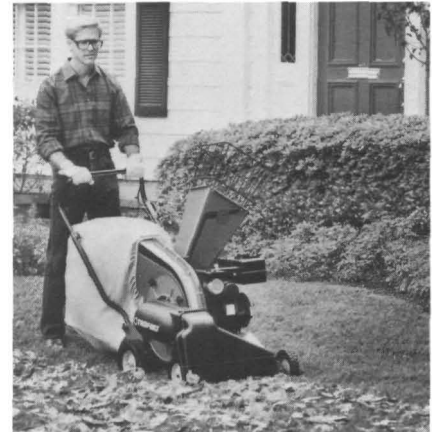
Photo 3-3: Vacuum Snout permits walk-behind vacuuming operation.
