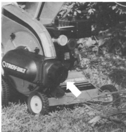
Photo 3-6: Vacuum Inlet Cap allows additional power for chipping operations.
