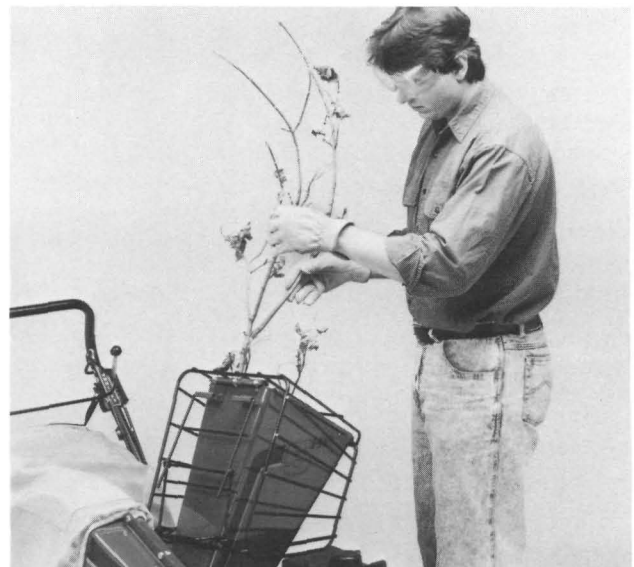
Photo 4-15: Using the chipper with the chute extension in the folded position.
