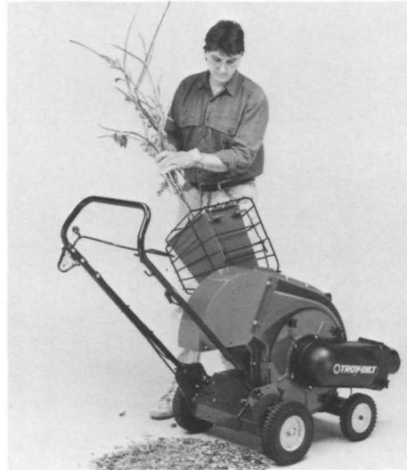
Figure 4-17: Stay away from the discharge deflector area when feeding the chipper without the collection bag installed.
