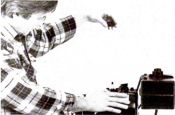
(Photo 2-7) On 5 HP Tecumseh engines, remove oil dipstick from oil fill tube, then add 19 ounces of motor oil using a clean funnel. Fill to "Full" mark on the dipstick. Do not overfill!
