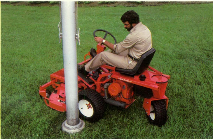
Pro Master-50 demonstrates 0° turning radius.
