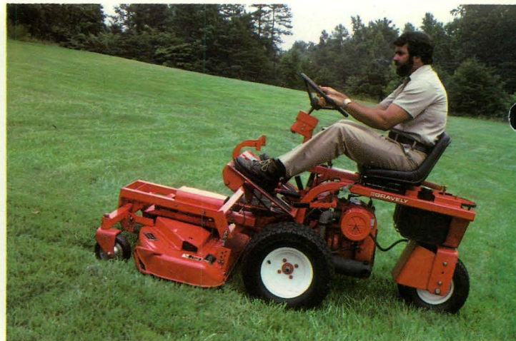
Hinged frame design delivers added traction on hills.
