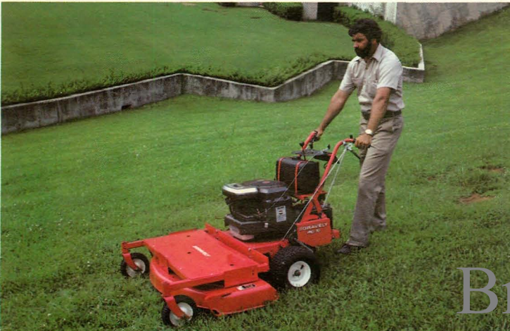
Wide spaced wheels provide hillside stability.
