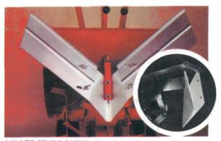
HILLER/FURROWER: The Hiller/Furrower hills corn, potatoes, etc. and helps to kill weeds in rows and between plants as it hills. Remove Hiller wings (no tools needed) and use Furrower alone to dig trenches for irrigation, drainage or trench composting (burying organic matter and kitchen leftover for improving soil). Makes furrows to plant potatoes, corn, asparagus, etc. Furrows to 8" deep, hills to 8" high.
