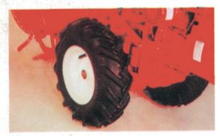
**BAR TREAD TIRES AND RIMS:** Especially helpful when extra traction is needed in loose, light, and sandy soils. Good for use with dozer blade, too. You can have your tiller equipped with these bar tread tubeless tires and rims (which most farm tractors also have). In place of diamond tread tires which are standard equipment.
