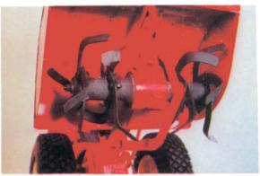
**BOLO TINES:** These are truly the all purpose Tines and are the type furnished on all new Troy-Bilts as standard equipment. For tilling in sod, weeds, cover crops, composted material as well as for seedbed preparation, tilling and cultivating. Their swept-back "bolo" design sheds excess matter and prevents most tangling of roots, grass and vines. Unlike many other tillers, each individual tine is replaceable. Bolos till 6-8 inches deep. #01 Standard equipment on Horse and Pony models.
