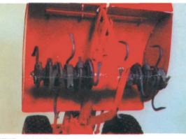
**POINTED PICK TINES:** Best choice of tines for especially tough, rocky, heavy clay, gumbo, or hardpan soils. Their springy "picking" action dislodges stones and breaks up hardpan. Tills up to 8 inches deep but tends to ball up in tall or thick grass, weeds and other organic matter. These tines do not fit in bolo holders.
